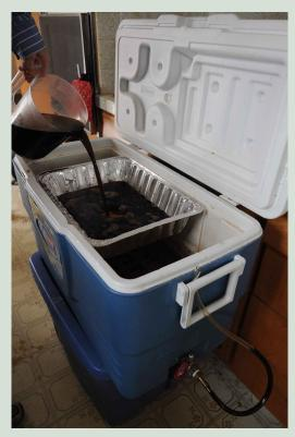
The wort is gently poured into the tin and allowed to drain through the nail-sized holes.
