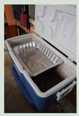
Before the wort is poured back into the mash tun, a \$4 cooking tin with about 50 holes is placed on top. The tin rests perfectly on the upper-ridges of the cooler.
