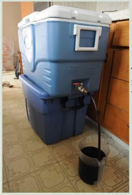
The first step of a standard pumpless vorlauf is to collect a few quarts of wort. The first few quarts are always cloudy with protein and grain debris.
